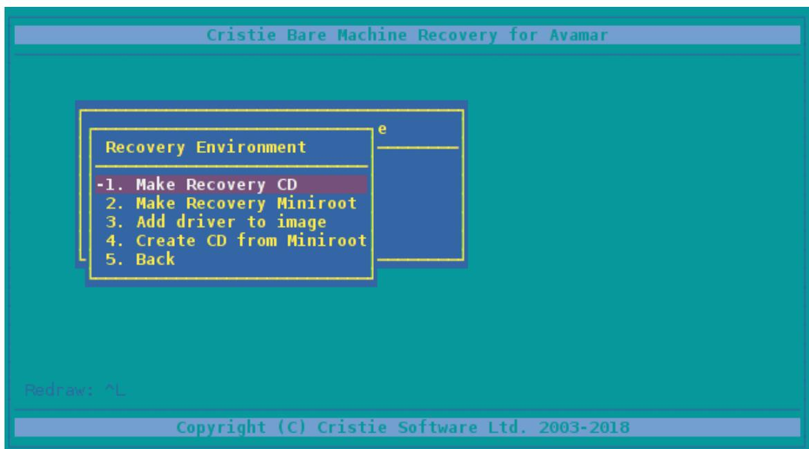
The first step is to create a recovery CD or PXE/Jumpstart bootable image. This is an image that can either be burned to CD to boot the recovery environment, or extracted to create a network boot environment.
