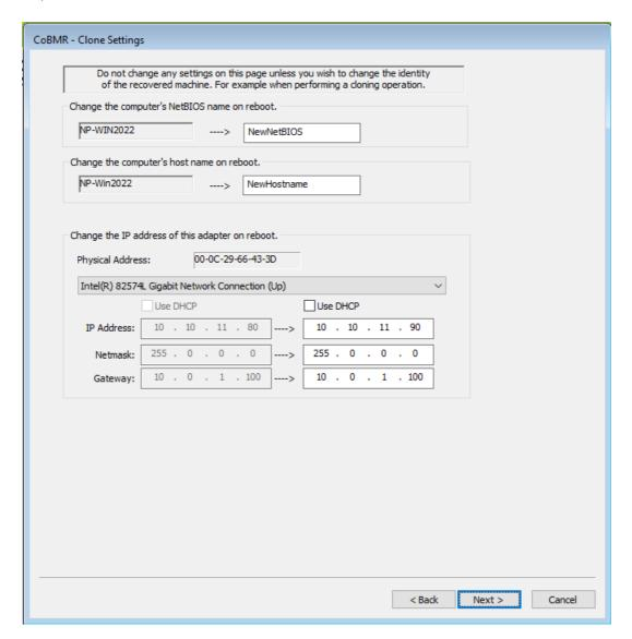
You may change the IP address for each NIC interface independently. NICs that are currently connected to a network are tagged with (Operational).
