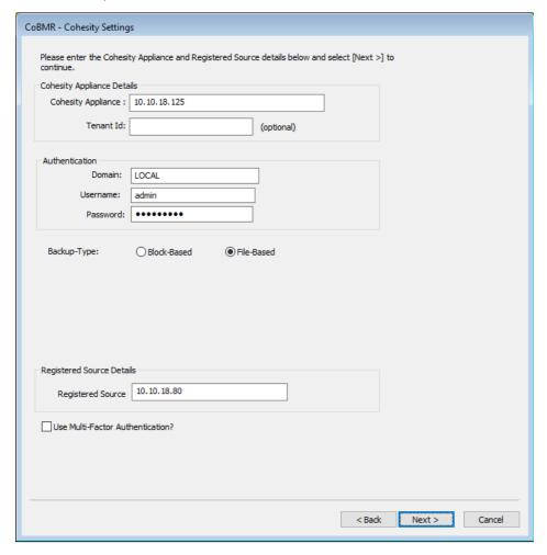
For **Registered Source** enter the IPv4 address or the name of the registered source, which must match the address or name used to originally register the source on the server. Enter a **Tenant Id** if required.
