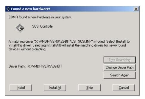
If you are satisfied that the found driver path is correct, click on **install** and the driver will be installed. The device scan will continue and may find, for example, other mass storage or network devices. Follow the steps above to install.
