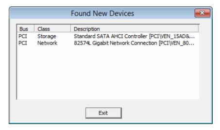
Ensure the specified path or paths contain the correct 64-bit drivers for the dissimilar machine. At the end of the DR sequence, the specified paths will be searched for the missing drivers and automatically injected into the recovered system.
