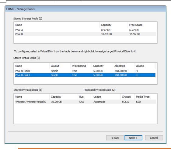
Note: There are some constraints on this configuration. For example, it is not recommended to have fewer or more physical disks mapped to your target virtual disk compared with the original source configuration.
