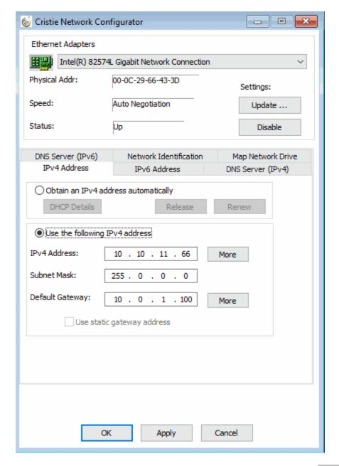
Set the new IP address, subnet mask and gateway IP address. The More button will allow the system to have more than one static IP address. Click on Apply to confirm the settings for the selected adapter.
