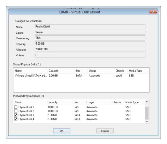
In the example above the 2 target physical disks that makeup the original virtual disk are selected. Note the proposed disk count is now non-zero.
