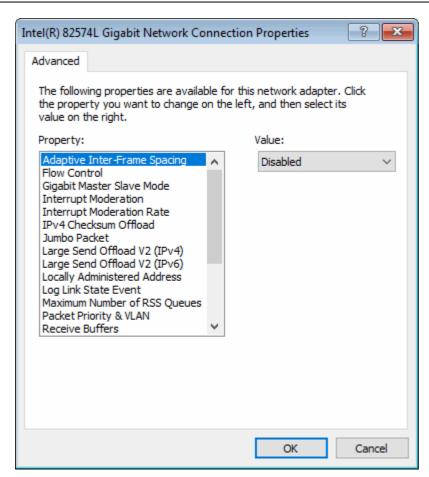
To change the NIC speed or duplex setting, select the corresponding Property from the dialogue and then select the required value from the Value drop down box as shown below:
