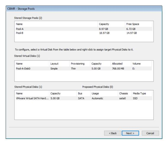
The pool configuration requires you to map the original pool/virtual disk configuration to the physical disk layout detected on the target. This may have more or fewer disks than the original so this re-mapping needs to be done manually.
