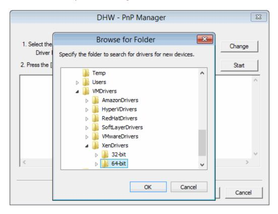
In the example above, the driver search path is changed to the VMware drivers on the WinPE boot CD. Begin the PnP driver detection by clicking Start.
