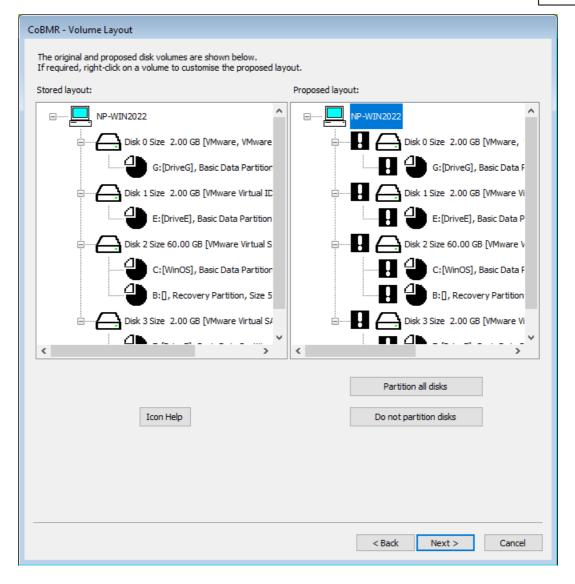
The left-hand panel of the dialogue shows the original disk layout and partitions. The right-hand panel shows how the recovered disks will be partitioned after the recovery.
