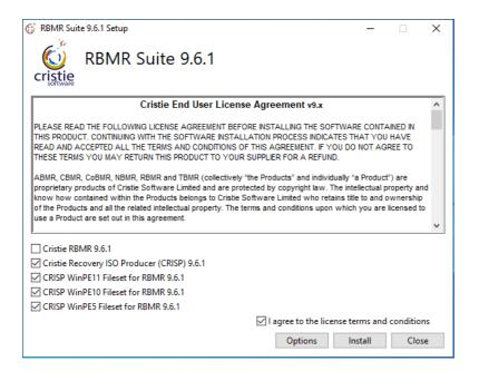
There is one option that can be configured prior to the installation. Click Options to open the options dialogue. You may then select a different installation folder. The VA fields are not relevant for the Install of CRISP and the fileset options.
